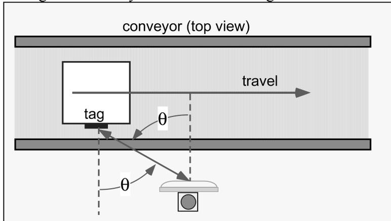
How does the read zone change, assuming that range is proportional to the power (voltage<sup>2</sup>)? How long does the tag spend in the read zone?
