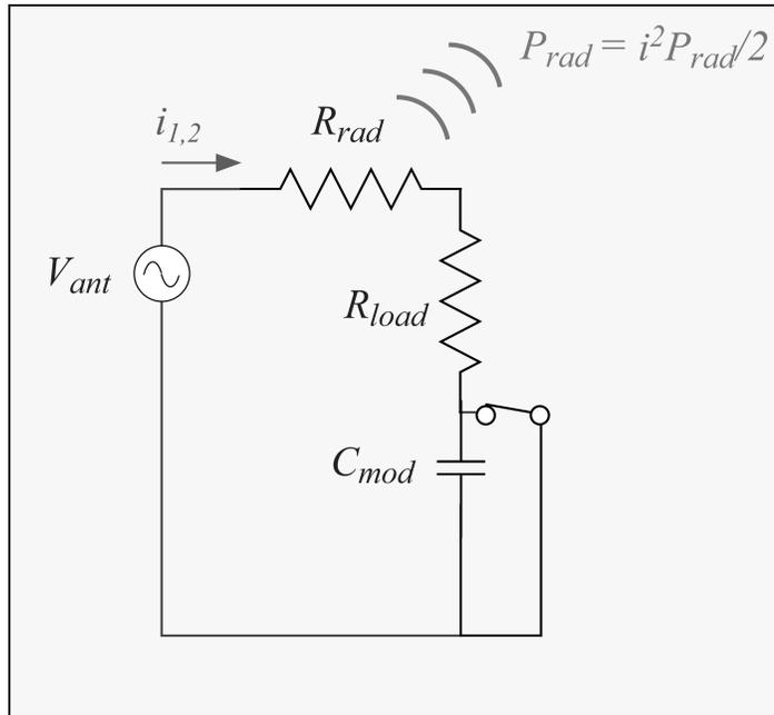
Find the power absorbed in the load in the modulated state as a fraction of the available power  $P_{av}$ .
