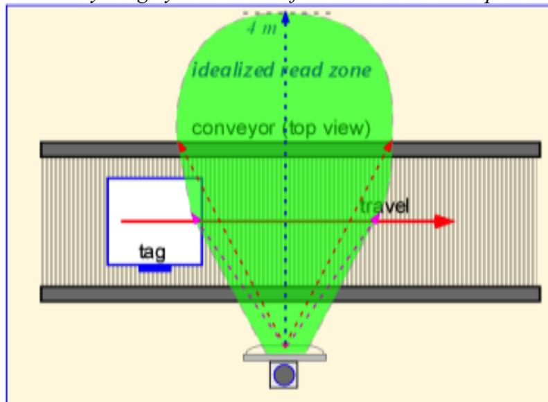
*In the idealized-read-zone approximation the time in the read zone is reduced by a factor of  $\sin(35^\circ)/\sin(45^\circ) \approx 0.8$ , so the time becomes about 0.65 s.*
