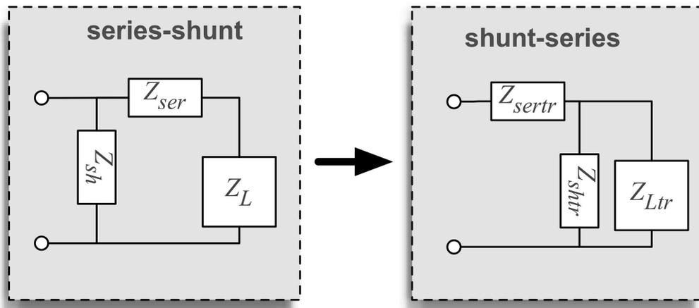
If this can be done, it has to work for the two limiting loads: an open circuit and a short circuit ( $Z_L = 0$  and  $\infty$ ). Using the formulas for series and parallel impedances (Appendix 3), we can show:
