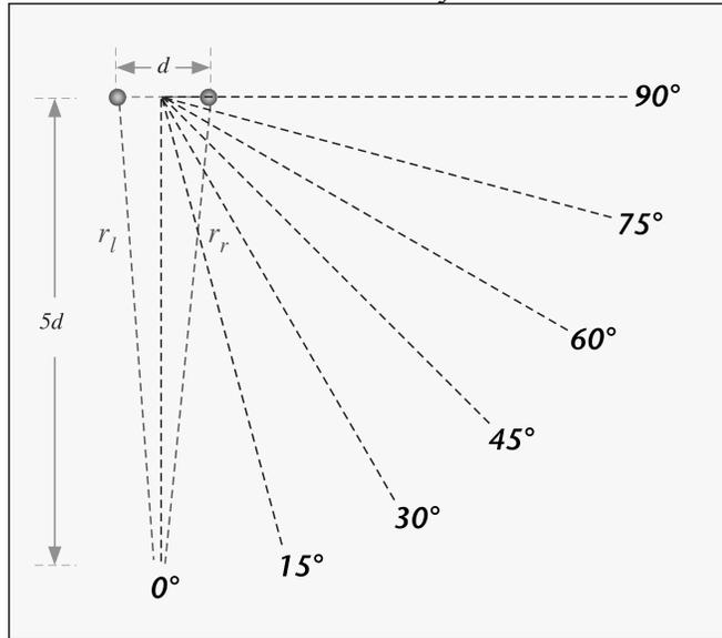
Treating  $5d$  as equal to  $\infty$  (and if you can do this without a second thought, you have a future in politics), measure the distances  $r_l$  and  $r_r$  from the two array elements to the end of the inclined dotted lines shown in the figure and record them, and their difference, below. (Use a ruler on paper, or use the digital version of the figure on the CD.)
