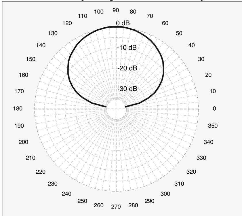
Extract the 3-dB and 6-dB beamwidth. *The 3-dB beamwidth is about  $65^\circ$  and the 6-dB beamwidth is about  $90^\circ$ , as shown below.*
