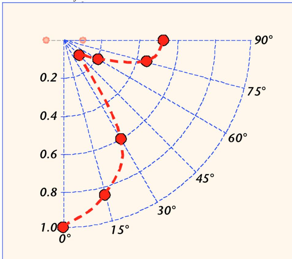
*You can see that there's a null in the pattern. This occurs when the distances to the two array elements differ by half a wavelength (i.e. when  $\delta=0.75$ ), as in that case the signals from the two elements arrive exactly  $180^\circ$  out of phase and cancel. So this array transmits mainly in the broadside direction; the endfire electric field (along the array axis) is reduced by about a factor of 2.*
