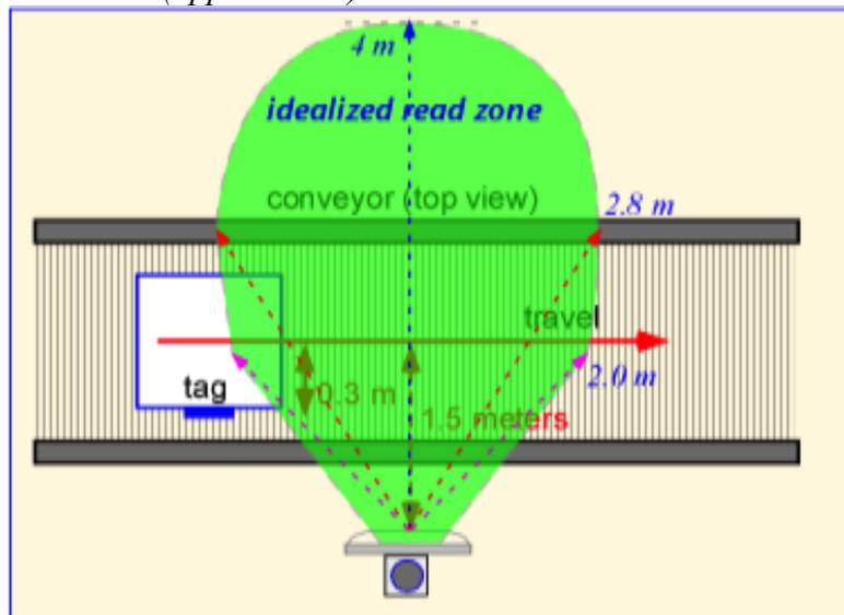
Assume tags are offset towards the antenna by 30 cm relative to the centerline of the conveyor, and that the cartons move along the conveyor at 3 meters/second. How long does a tag spend in the (idealized) read zone?
